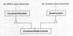
The solution involves a two-way class adapter ConstraintStateVariable, a subclass of both StateVariable and ConstraintVariable, that adapts the two interfaces to each other. Multiple inheritance is a viable solution in this case because the interfaces of the adapted classes are substantially different. The two-way class adapter conforms to both of the adapted classes and can work in either system.
