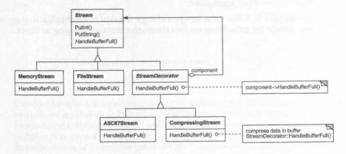
The Stream abstract class maintains an internal buffer and provides operations for storing data onto the stream (PutInt, PutString). Whenever the buffer is full, Stream calls the abstract operation HandleBufferFull, which does the actual data transfer. The FileStream version of this operation overrides this operation to transfer the buffer to a file.
