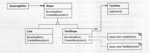
This diagram illustrates the object adapter case. It shows how BoundingBox requests, declared in class Shape, are converted to GetExtent requests defined in TextView. Since TextShape adapts TextView to the Shape interface, the drawing editor can reuse the otherwise incompatible TextView class.
