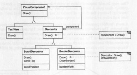
VisualComponent is the abstract class for visual objects. It defines their drawing and event handling interface. Note how the Decorator class simply forwards draw requests to its component, and how Decorator subclasses can extend this operation.
